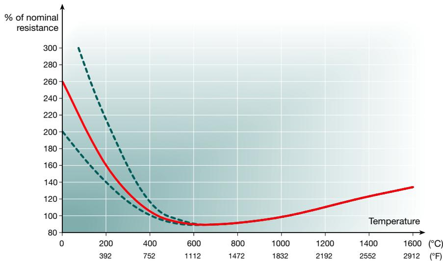
Fig. 4 Typical Resistance/Temperature Curve
