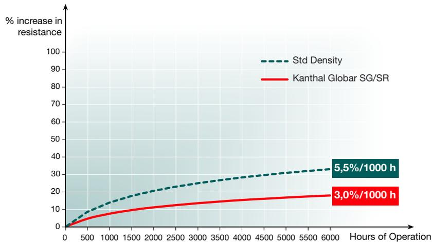
Fig. 3 Typical change in resistance with time at 1400°C (2552°F) (Continuous operation in an air atmosphere)
