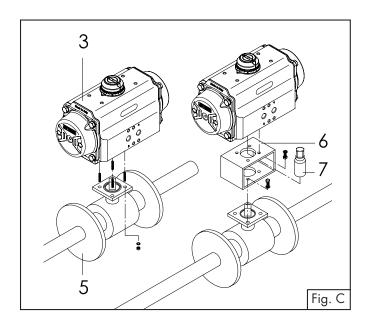
Before proceeding with the assembly of the actuator onto the valve, be sure that the actuator operates in the desired direction of rotation when pressurised and both actuator / valve are in the correct position.
