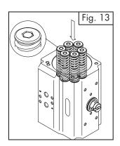
• Fit end cap o-ring seal (14) into the groove on both end caps.
