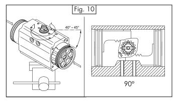
• Insert and press the two pistons (40) simultaneously inside the body (50) until the pistons are engaged, then rotate the body anticlockwise from top view until the stroke is completed.
